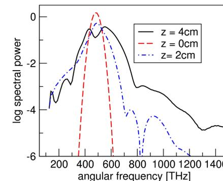
Propagation regime at high pressure is akin to femtosecond filamentation with the concomitant **supercontinuum** generation reflecting extreme nonlinear evolution.
