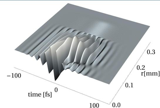
**Significant excitation of high-order modes.** Such modes have higher loss, but a superposition of them confines the total waveform to the interior of the waveguide. Actual loss is minimal. **gUPPE** correctly simulates this, but **ALMEX** cannot. Trailing edge of pulse in on-axis region depleted by generated plasma. Outgoing waves at  $r > 0.2\text{mm}$  absorbed by PML.
