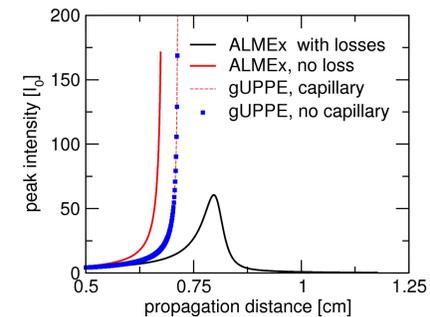
Self-focusing in the nonlinear regime in the waveguide causes an **explosion** of localized intensity above a critical power and at a critical propagation distance.
