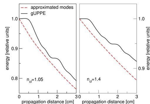
**Energy loss** experienced by initially collimated, pulsed Gaussian-beam with the beam waist smaller than the capillary inner diameter. **gUPPE** includes proper modelling of loss due to light leaking into the cladding. **ALMEX** incorrectly predicts loss since it is based on complex-valued propagation constants ascribed to orthonormal set of modes (spatially uniform loss).
